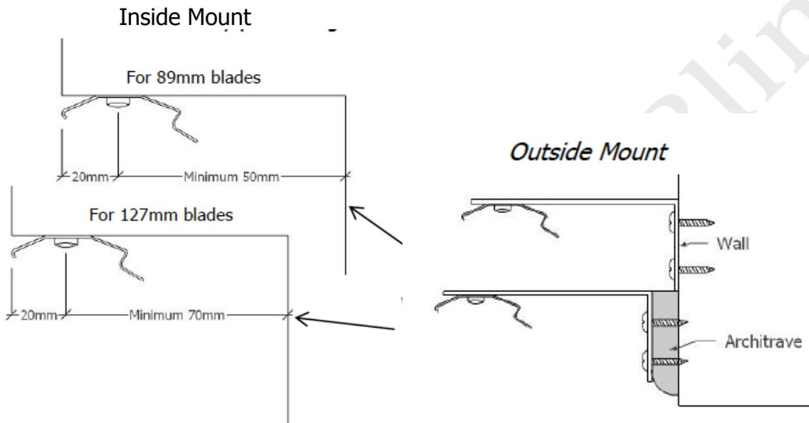
Position the brackets so that the blades clear the window frame or any protruding handles.
